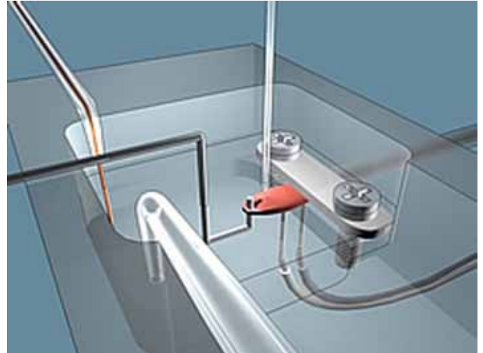
Schematic drawing of the experimental chamber of the papillary muscle set up
