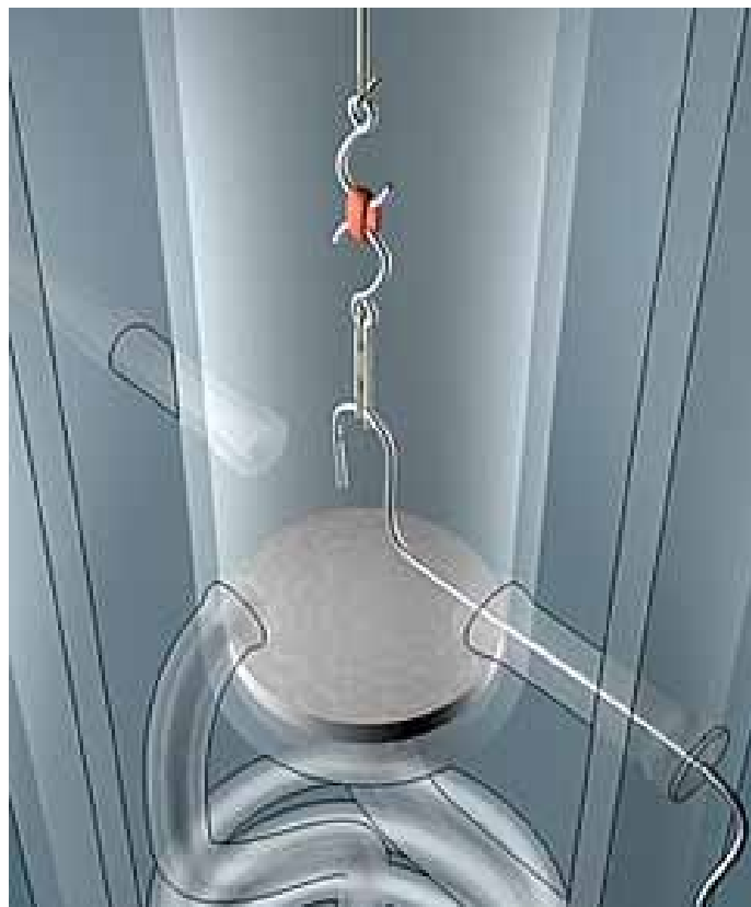
Schematic drawing of the experimental set up for measuring isometric contractions and field stimulation
